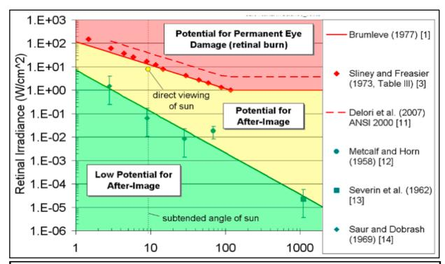
Solar Glare Ocular Hazard Plot: The potential ocular hazard from solar glare is a function of retinal irradiance and the subtended angle (size/distance) of the glare source. It should be noted that the ratio of spectrally weighted solar illuminance to solar irradiance at the earth's surface yields a conversion factor of ~100 lumens/W. Plot adapted from Ho et al., 2011.
